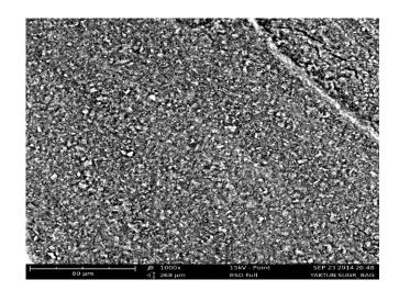
Figure 6: SEM image of the morphological analysis of carbonized sugarcane bagasse.
