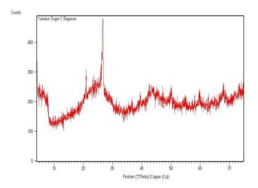
Figure 3: XRD pattern of sugar cane bagasse in selected MSW
