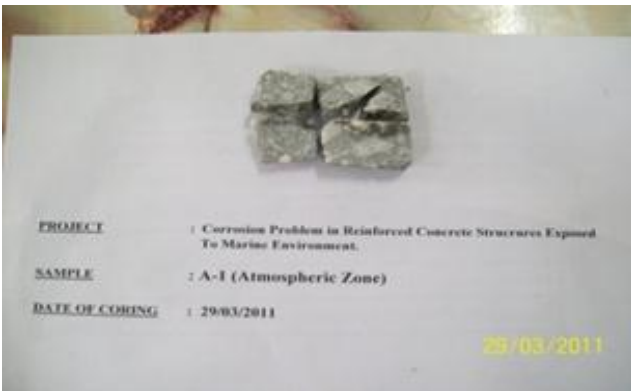
Figure3. Concrete particles from different zones for chloride content determination.
