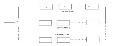
Fig.2.0 Reliability model of the battery bank at networks
