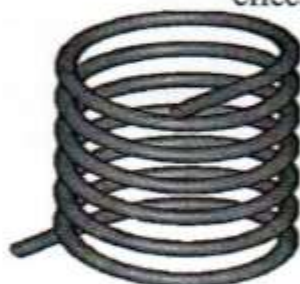
Plate 3: Coiled double pipe helical heat exchanger (Rennie, 2004)
