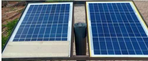
Figure 8: Normal image of 40W Polycrystalline module subjected to 20% horizontal shading.
