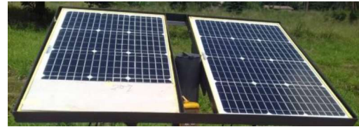
Figure 6: Normal image of 20% horizontal shading
