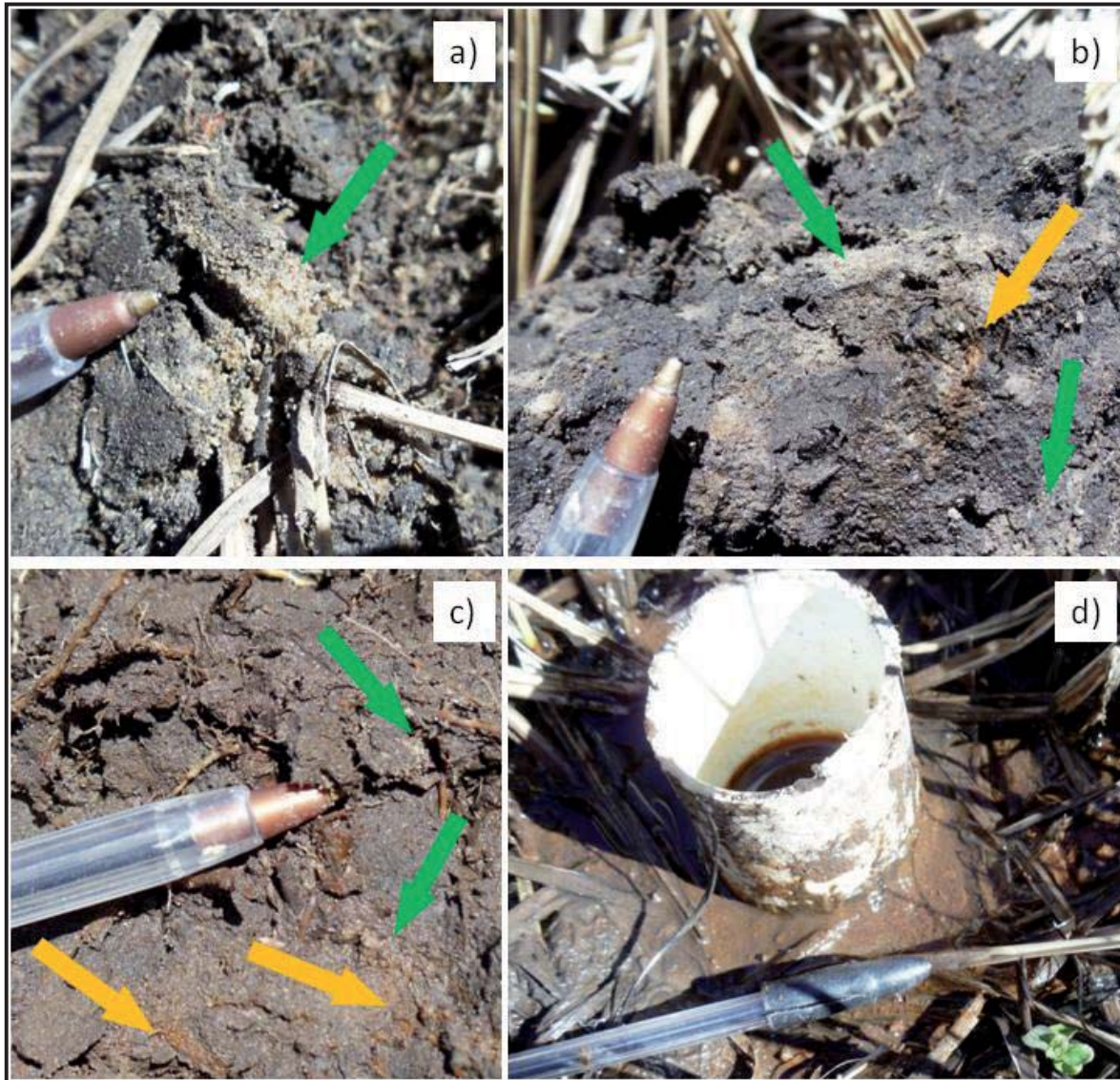
Figure 8: Related distribution of grey and red mottles. Green arrows indicate grey zones of Fe depletion (a, b and c), yellow arrows indicate zones of red zones of Fe accumulation (b and c) and d) ironoxide rich water flowing over the surface at HP10 of group 3.
