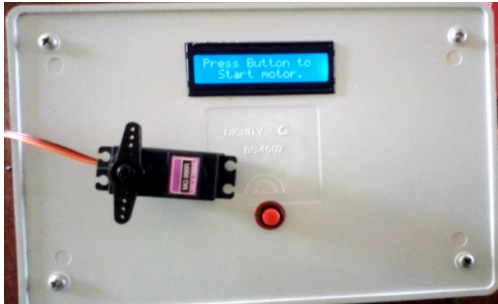
Figure c: Display with Instruction to Start Motor which is Still at Rest
