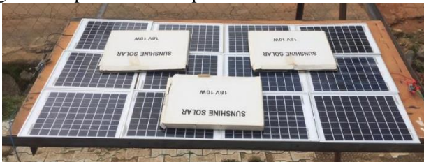
Figure 4: Setup for partial shading Condition
