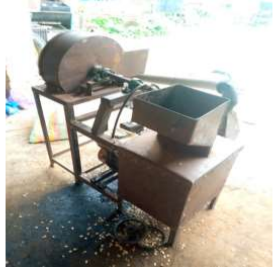
Fig 1: Pictorial side view of the melon shelling machine
