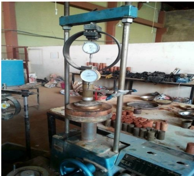
Figure 2: Unconfined compressive strength test
