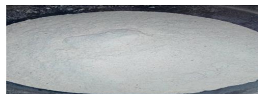
Plate III: Crushed Periwinkle Shell
