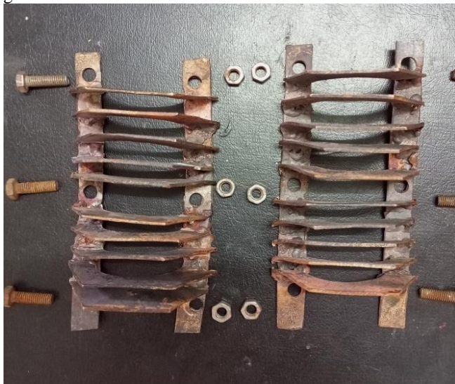
Plate III: Copper heat sink in dismantled form
