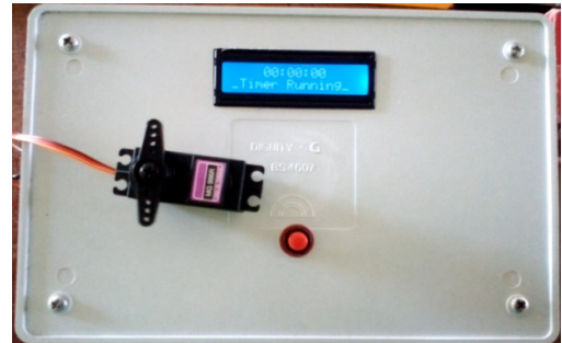
Figure g: Discharge Position, Motor back to Rest and End of Countdown
