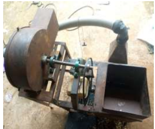
Fig 1: Pictorial top view of the melon shelling machine
