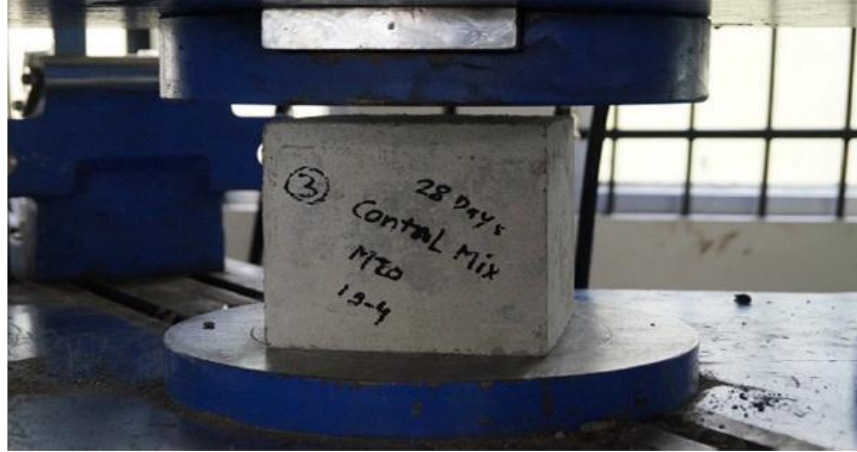
Figure 3: Compressive test of concrete cube
