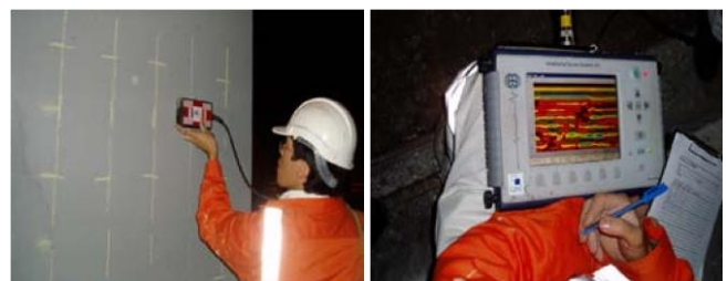
Figure 1 - Ground Penetrating Radar (GPR) testing utilising high frequency impulse radar
