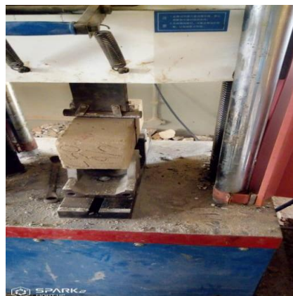
Plate 4: Flexural strength test
