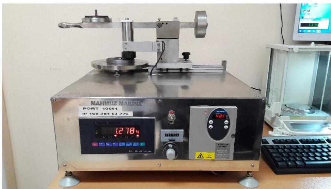
Figure 2.5. Pin-on-disc wear testin machine
