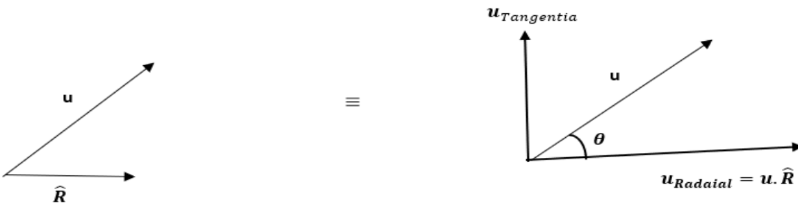
Figure 3: The geometry of the radial velocity component
