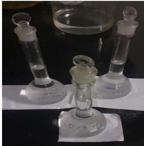
Figure 5 Standardization of Fluoride solution
