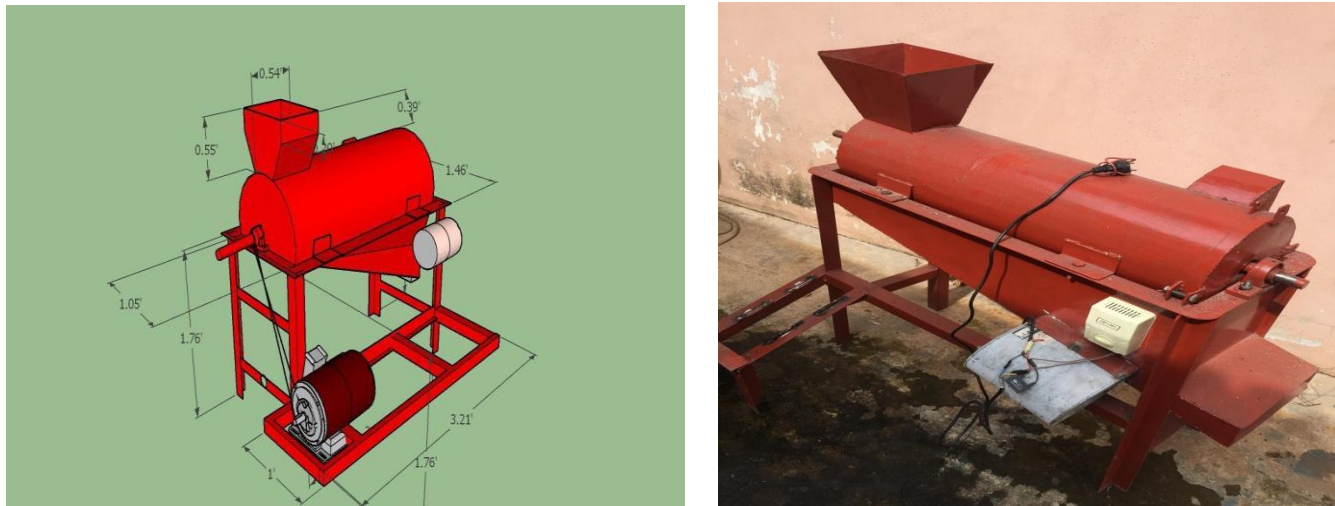
Figure 1: The Isometric View and the Developed Millet Dehulling Machine
