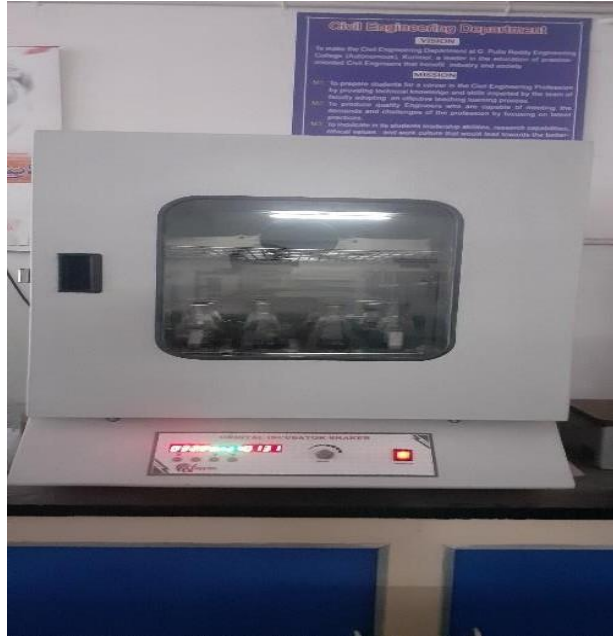
Figure 6 Orbital Incubator Shaker Apparatus
