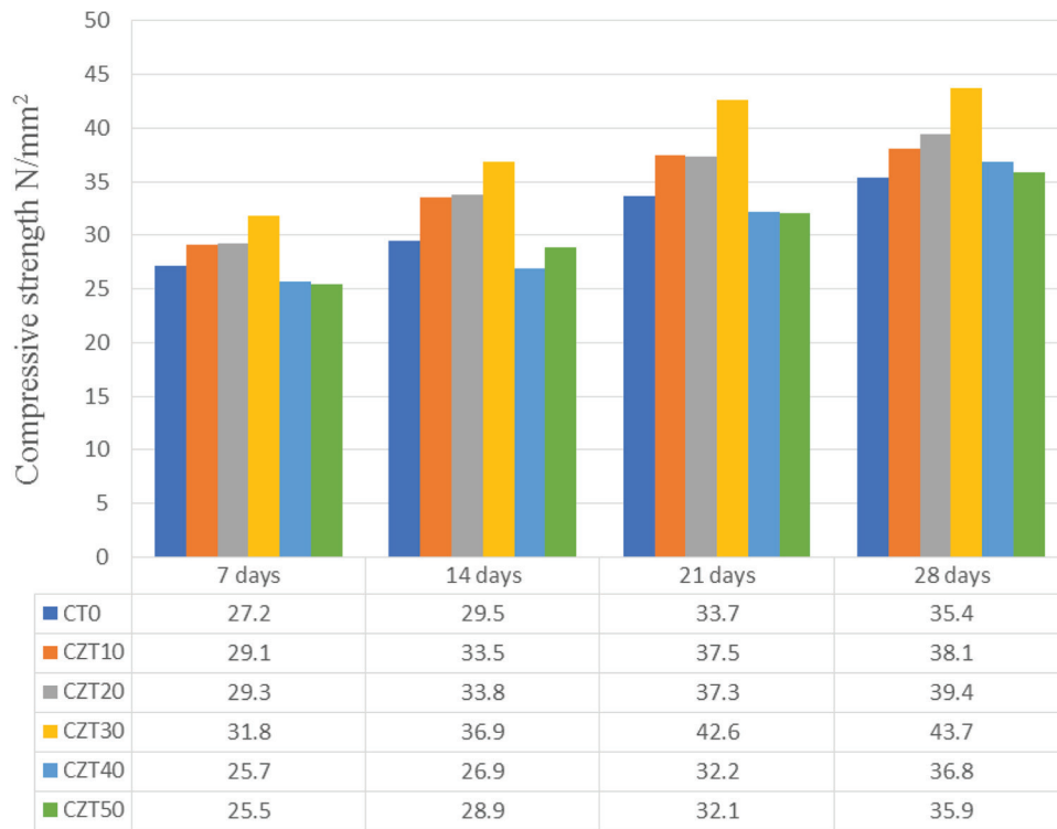
Fig. 10—Compressive strength of control and IOT concrete.
