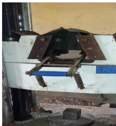
Plate 3: Compressive strength test
