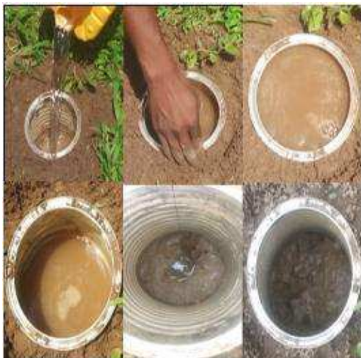
Plate III: Some of the Procedure involved in Infiltration Rate Experiment
