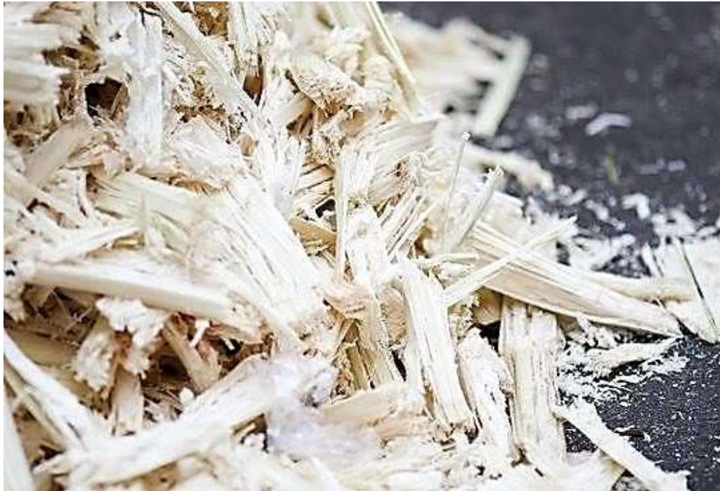
Figure 2.20: Sugarcane Bagasse Obtained from Sugarcane Stem after Extracting the Juice from the Stem Source: Alokika et al. (2021)
