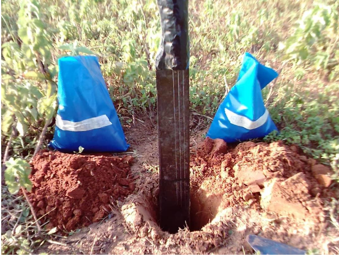
Soil Sampling at 0-15 cm and 15-30 cm with the aid of a cutlass at one of the location
