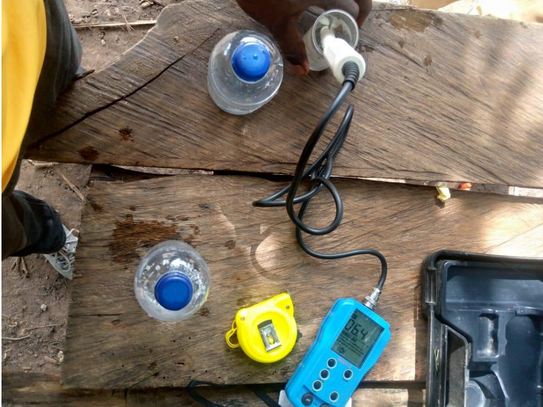
Taking the values of the various water parameters with the aid a Multimeter at one of the locations at Kudu
