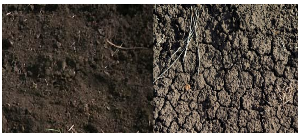
a. Dry state b. Wet state PLATE I: BLACK COTTON SOIL IN DIFFERENT FORMS
