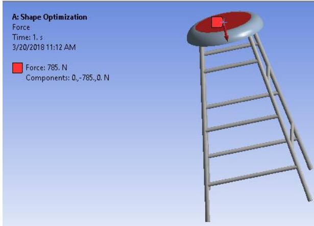
FIGURE 7: 785N LOAD CONSTRAINTS.
