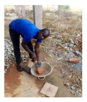
XI Abrasion test of the brick
