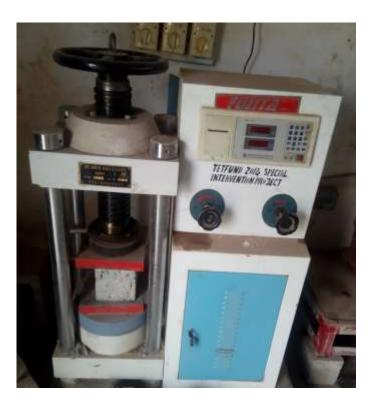
Plate II Compressive strength test machine.
