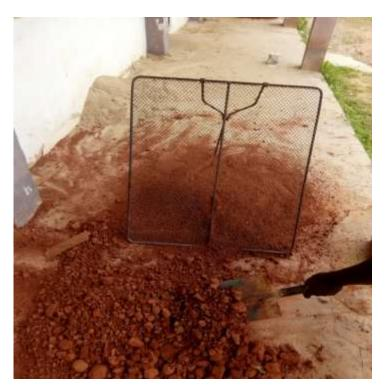
Plate V: Sieve lateterite using 5mm net
