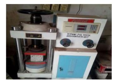
**Plate II: Compressive Strength Test Machine**
