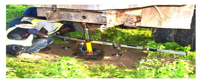
Figure 3. Conventional Plate load test.
