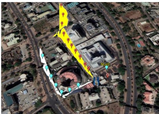
Figure 3: Simulation environment with a LOS and NLOS scena
