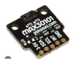
Figure 5: MAX30101 HR and BP sensor
