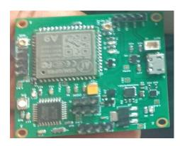
Figure 12a: HR/BP monitoring device (Front view)
