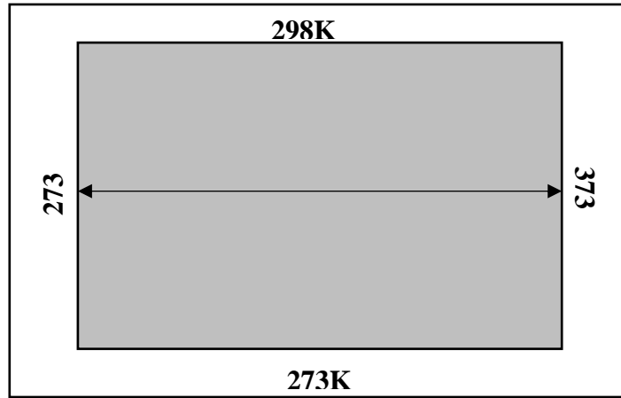
Figure 1: A Metallic plate with fixed Temperature
