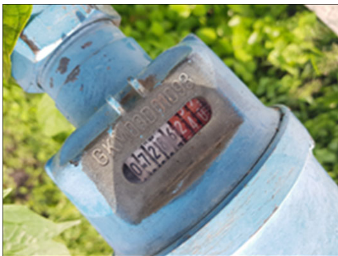
Fig. 37.3 Volumetric meter capsule reading
