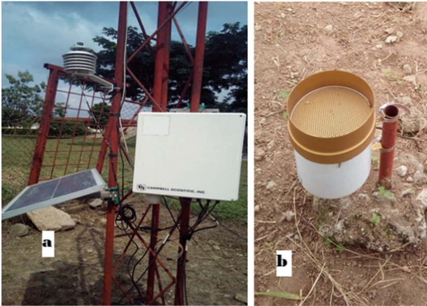
Fig. 36.1 a The TRODAN weather station (Campbell data logger and solar panel). b Tipping bucket rain gauge
