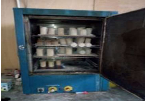
Fig. 4: Oven drying of the Briquettes
