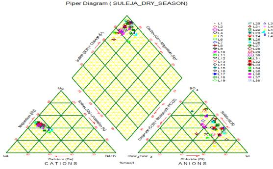
Figure 2: Hydrochemical Characterization of groundwater of Suleja Plotted on Piper Trilinear diagram for the dry season.
