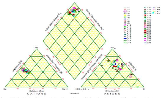
Figure 3: Hydrochemical Characterization of groundwater of Suleja Plotted on Piper Trilinear diagram for the wet season.
