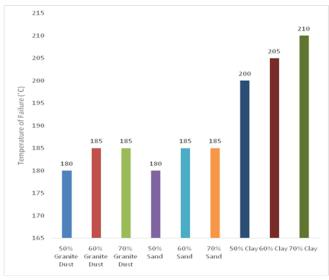
Figure 9: Comparison of failure temperatures of pavers from varying ratio of Plastic/geological materials
