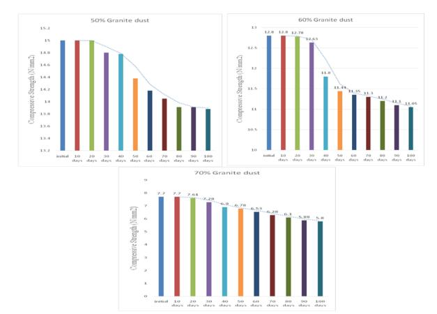
Figure 4 a-c: Chart of compressive strengths of pavers made of granite and plastic additives in different ratios a: Granite/Plastic=50/50, b: Granite/Plastic=60/40) and c: Granite/Plastic=70/30 on activation with weak sulphuric acid for between 0-100days.
