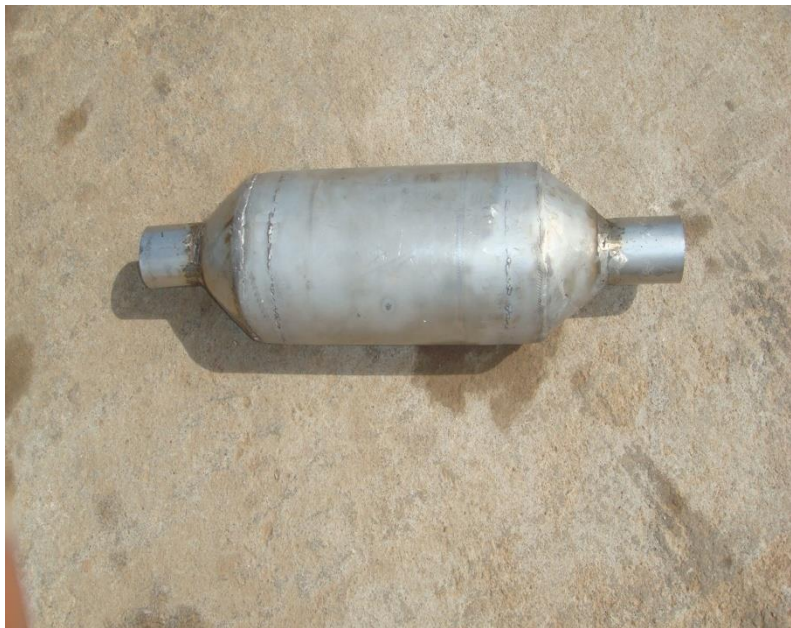
Plate I: The developed exhaust with 70mm inlet and outlet truncated conical sections
