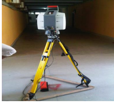
Figure 3: Showing the set up of the instrument, after connecting the cable
