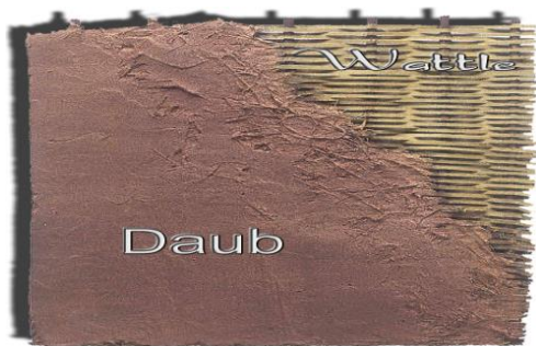
Plate III: Wattle and Daub construction.
