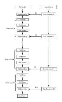
Fig 7: AES encryption process [16].
