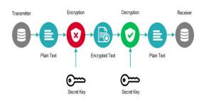
Fig 4: Working of encryption and decryption [8]
