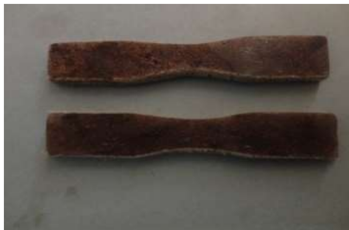
Plate IV: A typical wood polymer composite sample produced in this study.
