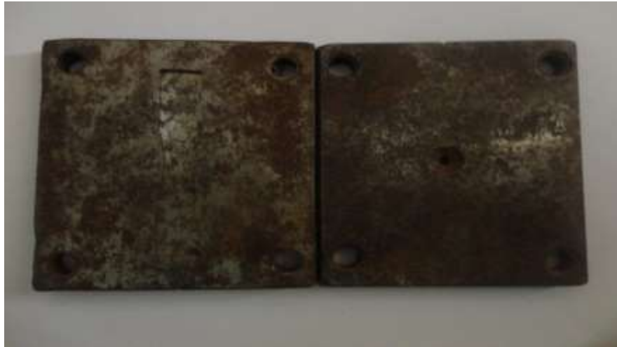
Plate III: The mild steel mould used for preparing composites of Daniella-oliveri wood dust in vHDPE.
