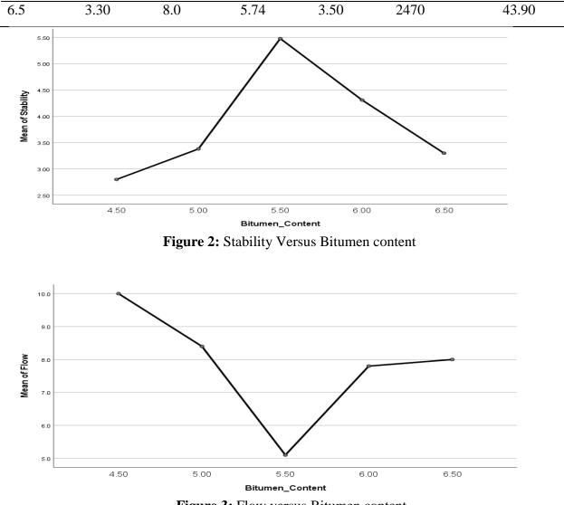
Figure 3: Flow versus Bitumen content
