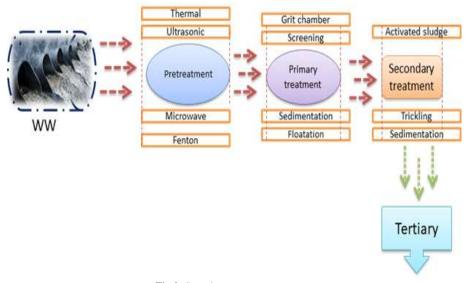
Fig 2: Steps in wastewater treatment
