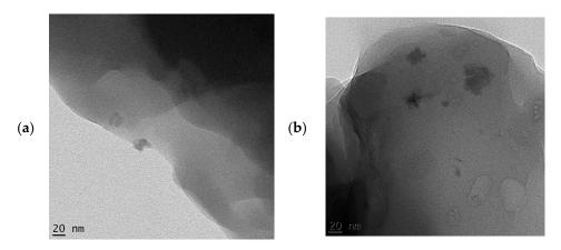
**Figure 3.** TEM micrographs of (a) cellulose nanofiber; (b) lignin fillers.
