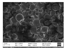
Figure 1. SEM micrograph of pure cassava starch film.
