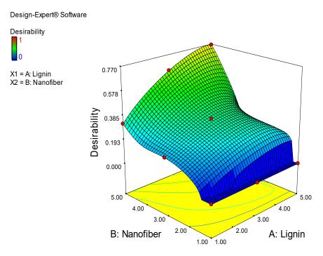
**Figure 5.** Desirability function of selecting the ideal film prepared.
