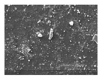
Figure 2. SEM micrograph of lignin-cellulose nanofiber-filled thermoplastic starch composite film.
