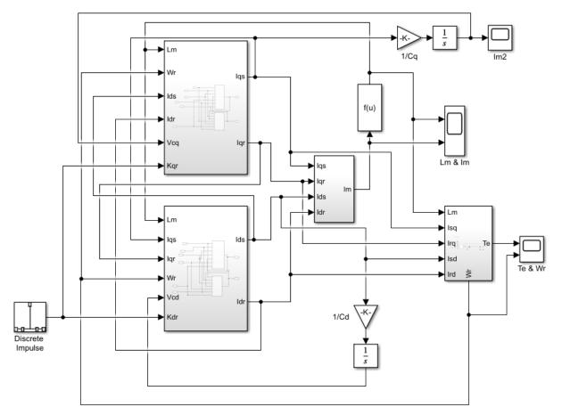
Figure 6: Simulation model diagram of SCIG.
