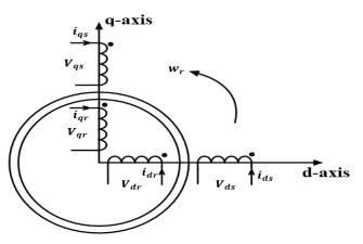
Figure 4: d-q representation of induction machine.
