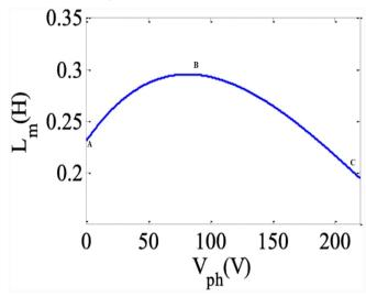
Figure 3: Saturation curve of Induction generator(Bendjeddou et al., 2021).
