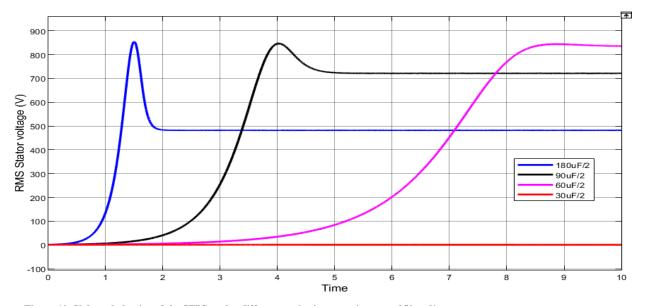
Figure 10: Voltage behavior of the SEIG under different excitation capacitance at 250 rad/sec.
