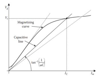
Figure 2: Saturation curve of Induction generator (Simoes and Farret, 2007)
