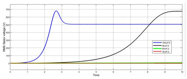
Figure 11: Voltage behavior of SEIG under different excitation capacitance at 200 rad/sec.
