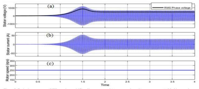
Figure 7: Excitation process at 180Uf capacitor and 250 rad/sec rotor speed (a) stator voltage (b) stator current (c) Machine speed.
