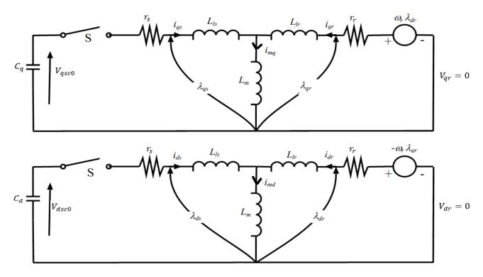
Figure 5: Equivalent circuit of capacitive SEIG.
