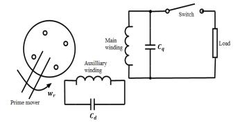
Figure 1: Schematic diagram of a capacitive excited and self-regulated induction single-phase generator.
