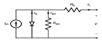
Fig. 6: Equivalent Circuit of PV Cell
