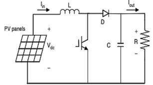
Fig 8: PV Boost Converter.
