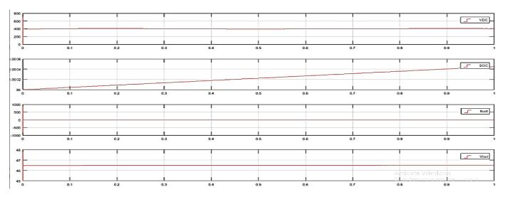
Figure 13: Bus Voltage, Battery SOC, Charging Current and Voltage
