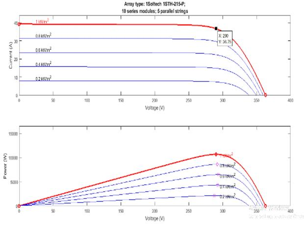
Fig 7: Isotech ISTH215P I-V and P-V characteristics.
