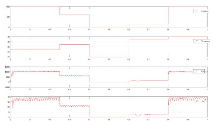
Figure 11: Solar Irradiation and Temperature Pattern, P&O MPPT Output Power and Current
