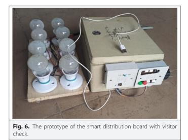
A part of the supply is used to power the DC fan through a rectifier circuit. Fig. 6 shows the implemented prototype of the smart distribution board with visitor check features.
