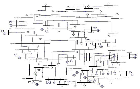
Figure 5: 52-Bus, 330 kV Nigerian Grid Single Line Diagram
