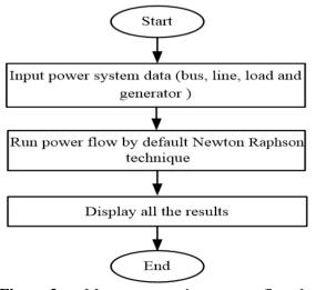
Figure 2: Matpower running process flowchart
