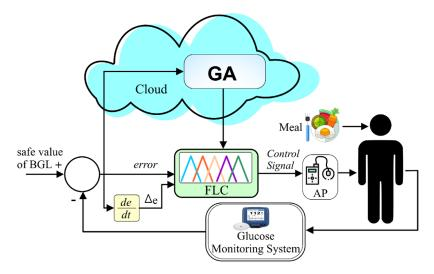
Fig. 4. Block diagram for the proposed fuzzy logic-based controller for type 1 diabetes patients
