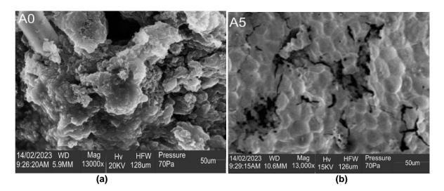
Fig. 4. Scanning electron micrographs of raw (a) and 3M H2SO4 activated (b) rice husk at 13000x magnification
