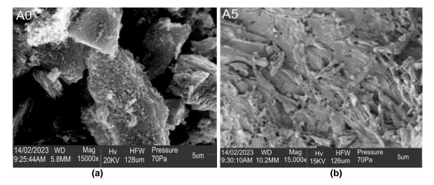
Fig. 5. Scanning electron micrographs of raw (a) and 3M H2SO4 activated (b) rice husk at 15000x magnification
