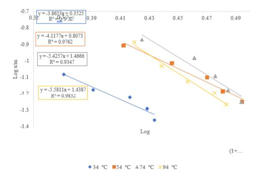
Fig. 19. Dubinin-Radushkevich isotherm plot for the bleaching process at different temperatures
