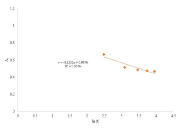
Fig. 15. Elovich kinetic model plot
