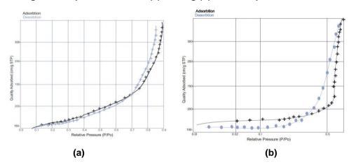
Fig. 7. Nitrogen adsorption BET linear (a) and log (b) isotherm plot of raw rice husk
