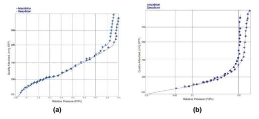
Fig. 6. Nitrogen adsorption BET linear (a) and log (b) isotherm plot of activated rice husk
