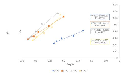
Fig. 18. Temkin isotherm plot for the bleaching process at different temperatures
