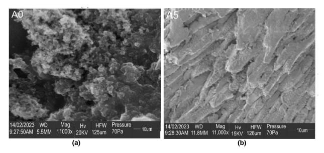
Fig. 3. Scanning electron micrographs of raw (a) and 3M H2SO4 activated (b) rice husk at 11000x magnification
