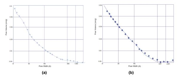
Fig. 8. BJH adsorption pore volume plot for the raw (a) and activated rice husk (b)
