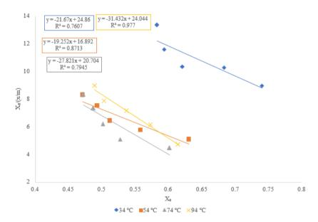
Fig. 17. Langmuir isotherm plot for the bleaching process at different temperatures
