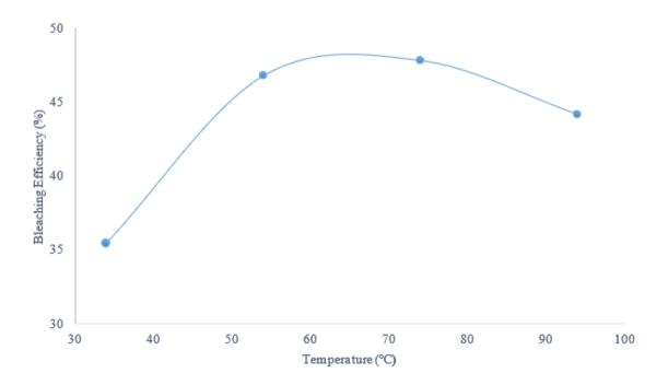
Fig. 10. Plot of bleaching efficiency against temperature
