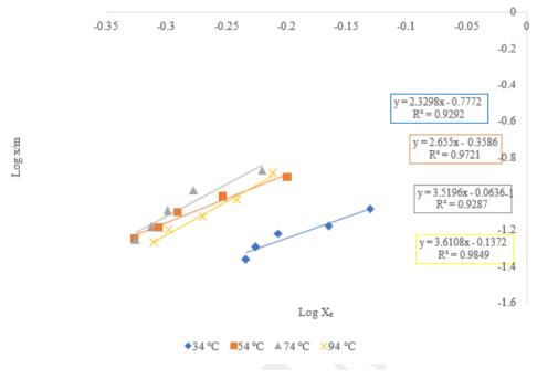
Fig. 16. Freundlich isotherm plot for the bleaching process at different temperatures
