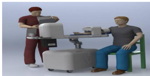
Fig. 3. Veebot robot drawing blood from a patient [33]
