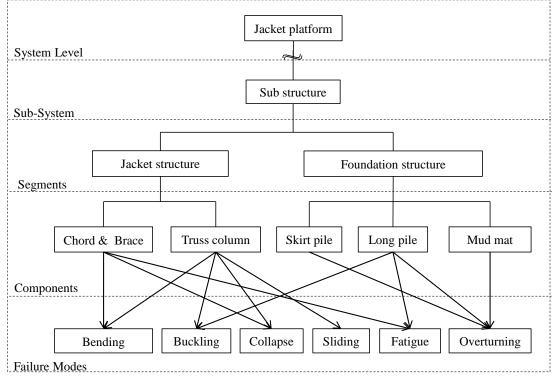
Fig. 2: Hierarchical structure for Offshore Wind Turbine Support Structure
