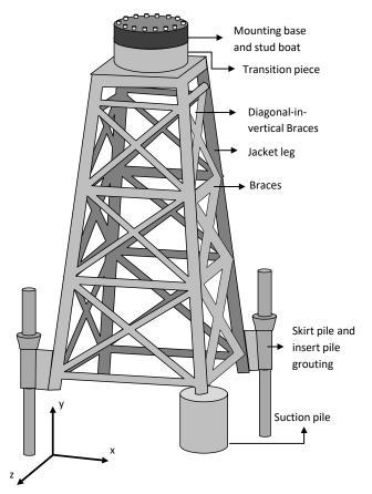
Fig. 3: Offshore Wind Turbine Support Structure
