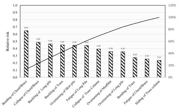
Fig. 5: Risk index of Failure modes
