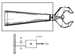
Figure Q1: 1 DOF Robot Arm
