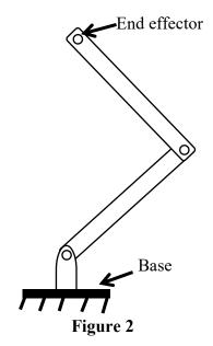
Figure 2 represents a 2 DOF serial manipulator. Using the Denavit-Hartenberg Notations,
