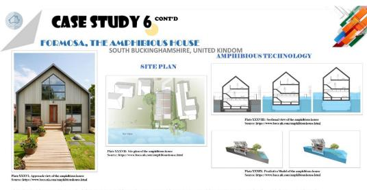
AN AMPHIBIOUS HOUSE, A BUILDING THAT RESTS ON THE GROUND WHEN CONDITIONS ARE DRY, BUT RISES UP IN ITS DOCK AND FLOATS DURING A FLOOD. THE HOUSE ITSELF SITS IN THE GROUND AND THE FLOATING BASE IS ALMOST INVISIBLE FROM THE OUTSIDE. THE GROUND FLOOR OF THE HOUSE IS RAISED ABOVE THE GROUND BY LESS THAN 1 M RATHER THAN BY ALMOST 2 M AS WILL BE REQUIRED IF IT WERE NOT AMPHIBIOUS.
