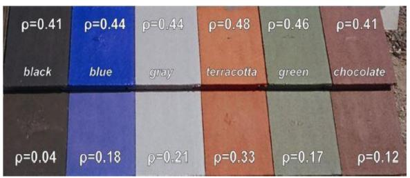
Figure 2.12. Cool dark colour roofs Source: (Chetan *et al.*, 2020).
