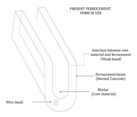
Figure 3.3: Existing Ferrocement Form (Plane bond)
