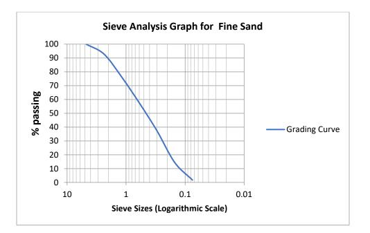
Figure 3.1: Sieve Analysis Graph for Fine Sand
