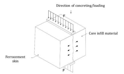
Figure 3.5: 2-D representation of specimen for plane bond testing
