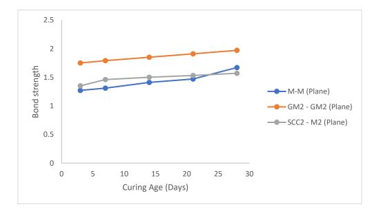
Figure 4.1: Bond strength versus curing Age for Plane bond specimens
