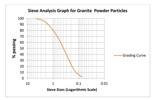
Figure 3.2: Sieve Analysis Graph for Granite Particle Sand
