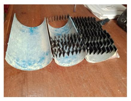
Plate 3.2: Layout of interlock test specimen preparation
