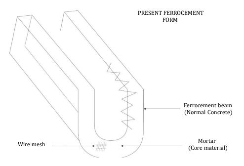
Figure 3.4: Experimental Ferrocement Form (Interlock bond)
