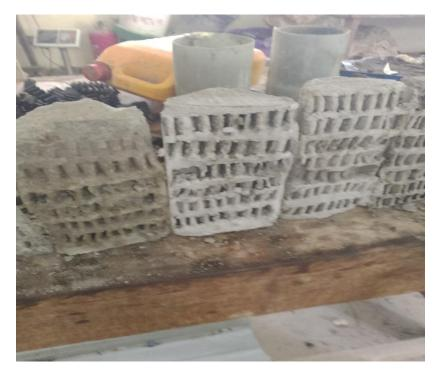
**Plate 3.3: Cast Interlock bond Specimens**
