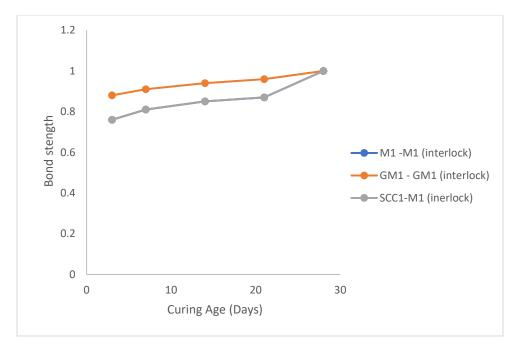
Figure 4.4: Relative bond strength versus curing Age for Interlock bond Specimens
