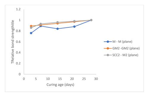
Figure 4.3: Relative bond strength versus curing Age for Plane bond specimens
