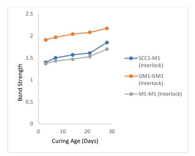
Figure 4.2: Bond strength versus curing Age for Interlock bond specimens
