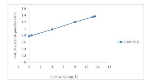
Figure 4.7: Volume of water to powder ratio versus relative slump for 30 % QD mix
