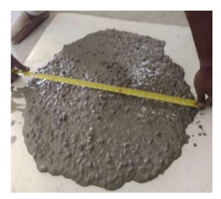
Plate III: Slump Flow Value of a Test Mix
