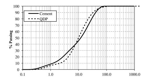
Figure 4.1: Particle size distribution of PC and QDP
