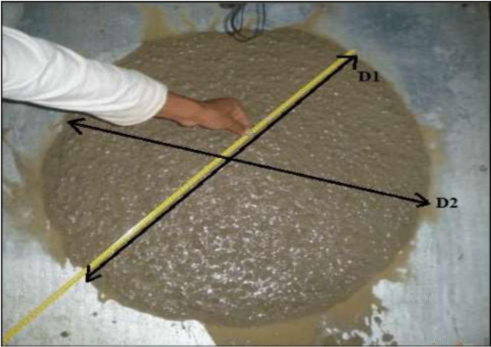
Figure 4.2: Slump flow values measured practically for Mixes tested.
