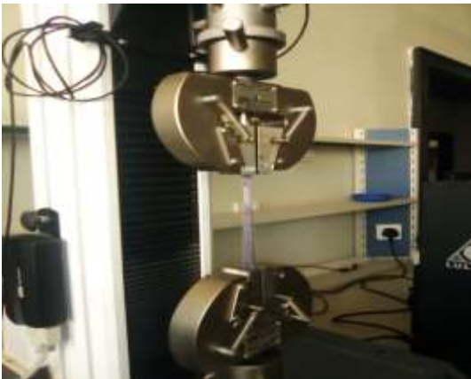
SAMPLE UNDER TENSION FOR TENSILE TEST
