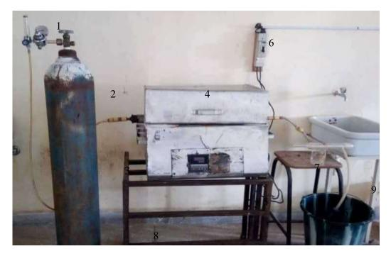
Plate V: Pyrolysis Experimental Set up
