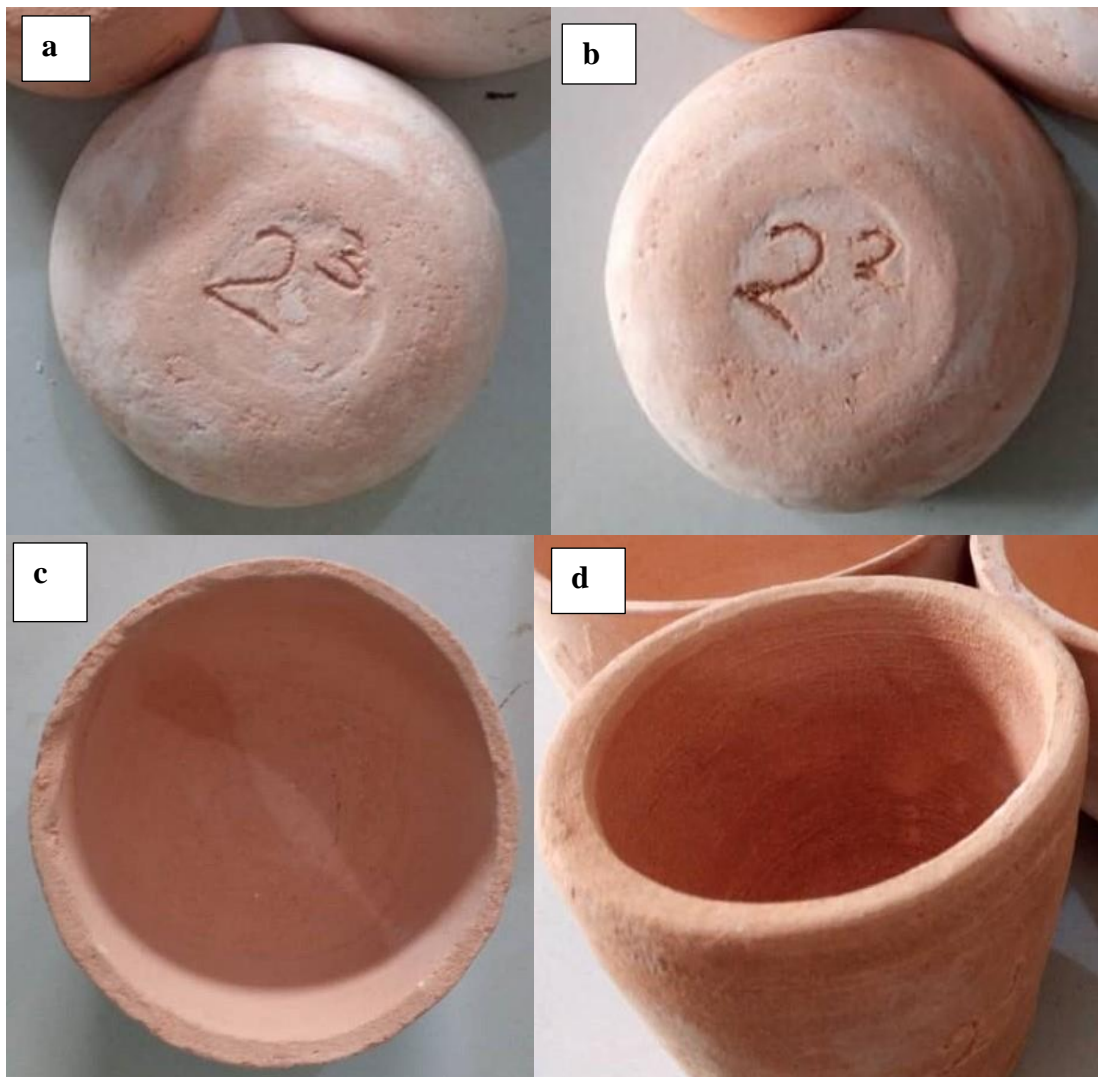
Plate XXI: (a). BKC/Ag/ZnO Filter Pot, (b). BKC/Ag Filter Pot, (c). BKC/ZnO Filter Pot and (d). BKC Filter Pot
